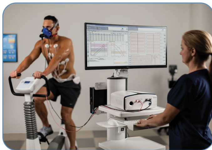
Figure 2. Vyntus™ CPX is an example of a CPET measuring device*.
